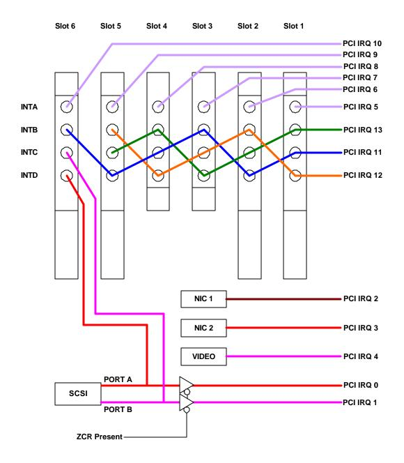
Figure 5. SDS2 PCI Interrupt Mapping Diagram
